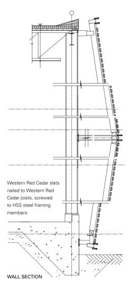
While the outward appearance of the pavilion is organic, with an undulating skin of Western Red Cedar slats, the underlying structure is rectangular and clad in stainless steel sandwich panels. An exterior framework of steel tubes forms the supporting structure for WRC joists, to which the more than  $4800\text{m}^2$  of WRC slats are fastened. The cedar skin is divided into radiating triangular panels, in a geometric pattern reminiscent of maple leaves.
