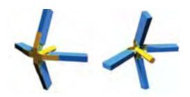
DETAIL OF STEEL SUPPORTING STRUCTURE FOR WRC CLADDING
