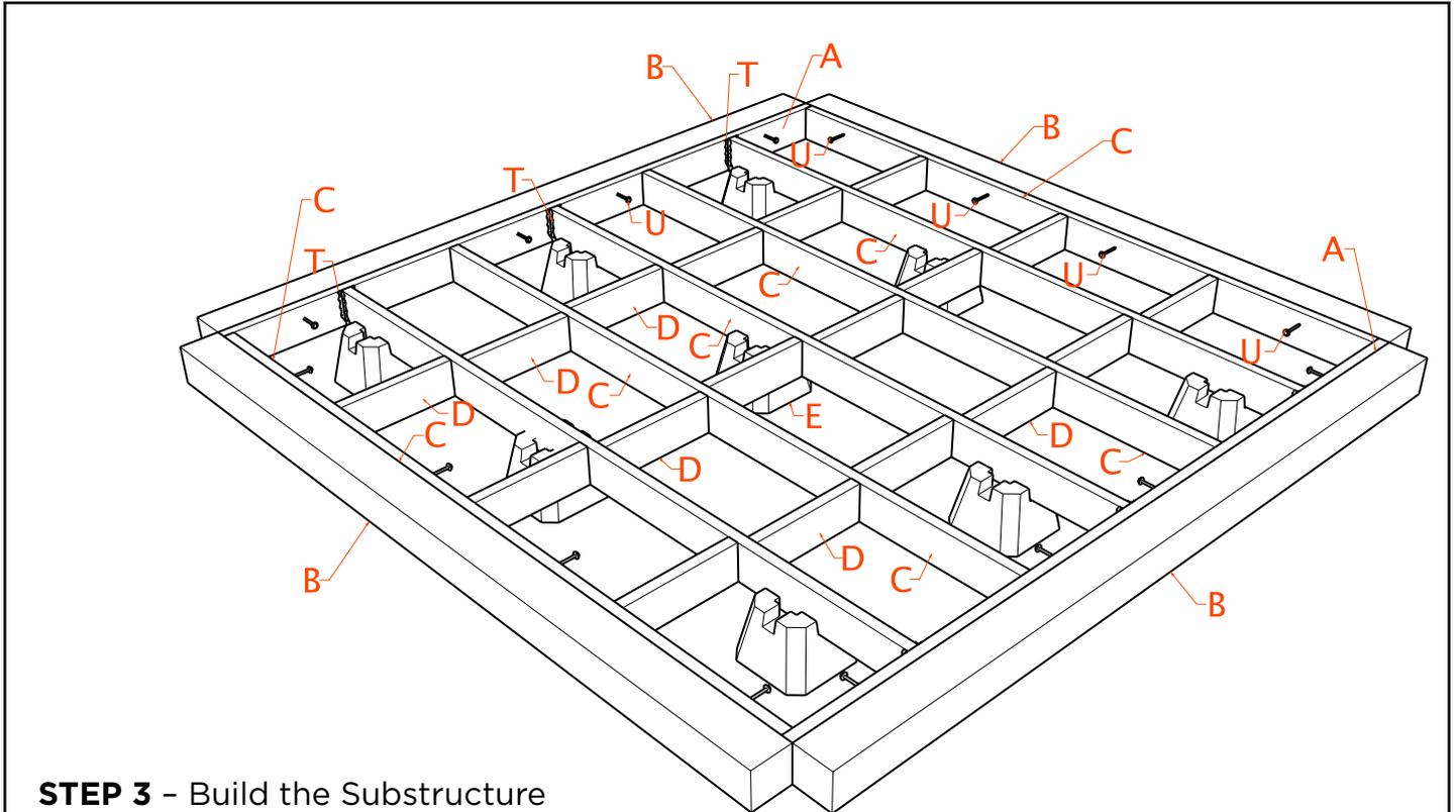
Insert three (C) 2 x 6 joists into concrete blocks. Attach both (A) rim joists with (T) joist hangers. Then attach remaining four (C) joists to frame. Fine tune fitting with a shim or cedar wedge and make sure it's square before attaching one (B) 6 x 6 rim joist to all four sides of the outer frame with (U) lag bolts and washers. Then secure structure by installing 18 (D) 2 x 6 bridge blockers in between joists.
